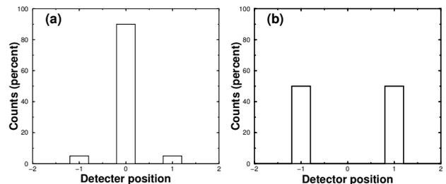
FIG. 5: Results that the detectors  $D+$ ,  $D0$  and  $D-$  are expected to show (a) without the detector  $D1$  and the Stern-Gerlach field in the path of particle  $A$ , and (b) with coincident counting with the detector  $D1$ . Here, detector positions  $-1, 0, +1$  correspond to the detectors  $D-, D0$  and  $D+$  respectively.
