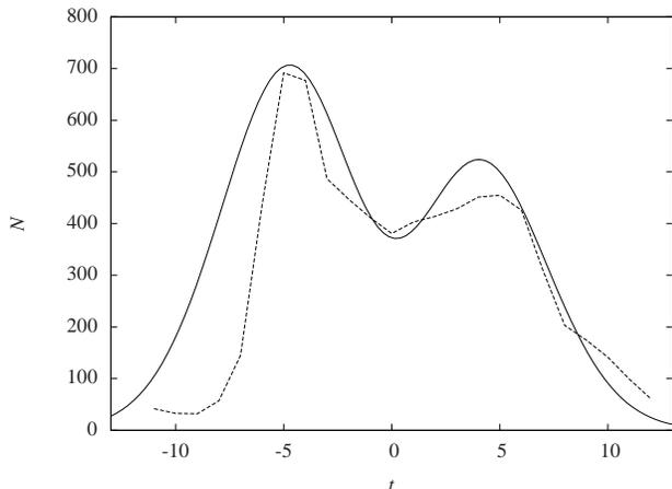
FIG. 1: Bimodal distribution of traffic flow due west. The vertical axis measures the volume of traffic,  $N$ , for a given time,  $t$  (scaled in hours). The horizontal axis has been scaled so that  $t = 0$  is set at midday, 12:00 hours. The dotted broken curve joins the real data points, and the continuous curve traces the model given by Eq. (2). The parameter values used for the fit are  $A = 44.0$ ,  $\mu = 8.53$ ,  $\lambda = 0.19$  and  $\beta = -0.09$ .
