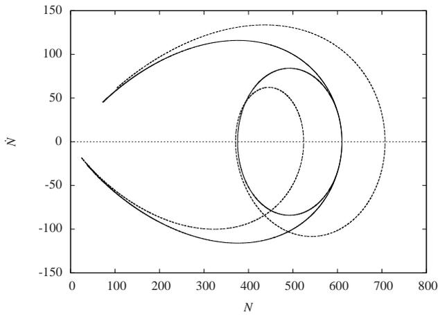
FIG. 5: Phase plot of the bimodal distribution of the traffic flow due west. Both the curves are plotted for the values of  $A$ ,  $\mu$  and  $\lambda$  used in Fig. 1. When  $\beta = 0$ , the resulting plot is shown by the continuous symmetric curve. When  $\beta = -0.09$  (as in Fig. 1), asymmetry sets in, as shown by the dotted curve.
