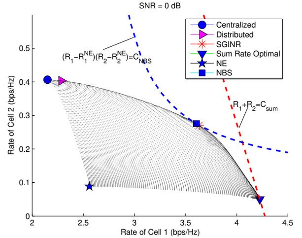
Fig. 2. The rate points of the multicell schemes and the Pareto boundary under a random channel realization, with  $(M, K) = (4, 2)$  and  $\text{SNR}=0$  dB.
