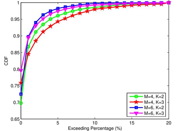
Fig. 3. The CDF of the excessive power percentage for the calculated downlink power vector with  $\text{SNR}=10$  dB.
