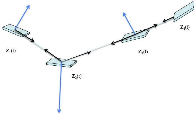
Figure 1: 4-parallelepipeds swimmer with all elastic forces and rotation forces about  $z_2(t)$  only.
