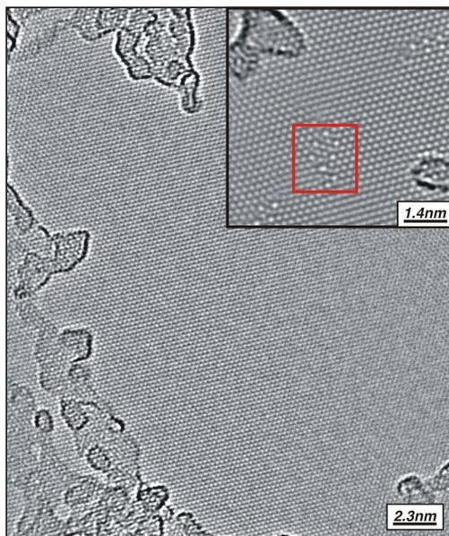
**Figure 4, Beam induced defects:** At 80keV the crystalline structure of graphene is stable at high doses but begins to demonstrate extensive defects left by knock-on damage (inset, red box) after comparatively low electron dose at 300keV ( $\sim 10^7 \text{ e}^-/\text{nm}^2$ ). Note that the inset area was imaged at 80keV after brief dose at 300keV.
