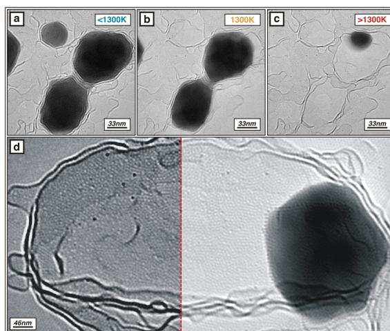
**Figure 7, Evaporation of gold particles by Joule heating across graphene:** (a-c) The gold particles melt during in-situ observation at temperatures of  $<1300\text{K}$ ,  $1300\text{K}$  and  $>1300\text{K}$  respectively, leaving behind an encapsulating carbon shell. (d) High-resolution image of the carbon shell. In the left part of the image, the underlying graphene lattice was removed by a Fourier filter and the contrast was increased. Adapted from [45, 46].
