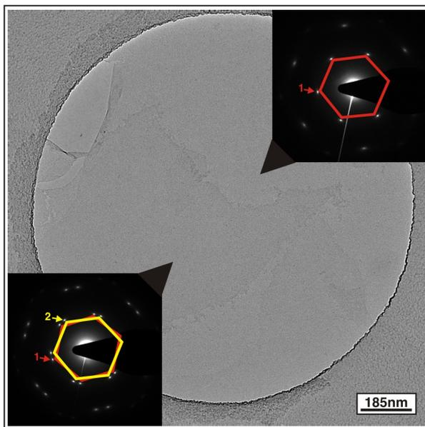
**Figure 2, The inadvertent stacking of graphene oxide layers:** An area of  $1 \mu\text{m}$  perforated amorphous carbon spanned by single (a) and double (a) layers of freestanding graphene oxide (defocus  $-2 \mu\text{m}$ , pixel size  $7.4 \text{ \AA}$ ) as indicated by superimposed hexagonal diffraction patterns corresponding to each layer (insets).
