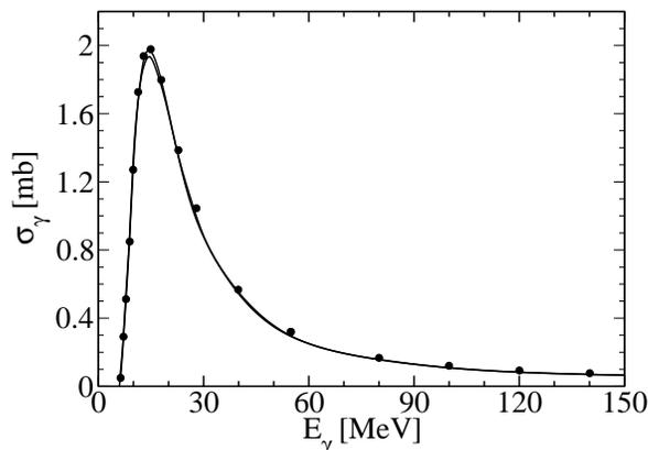
Figure 7: Results for the total  ${}^3\text{H}$  photoabsorption cross section with the AV18 potential from LIT/CHH (full) and Faddeev (dots) calculations in unretarded dipole approximation (the two curves represent the uncertainty of the inversion of the LIT); from Ref. [158].
