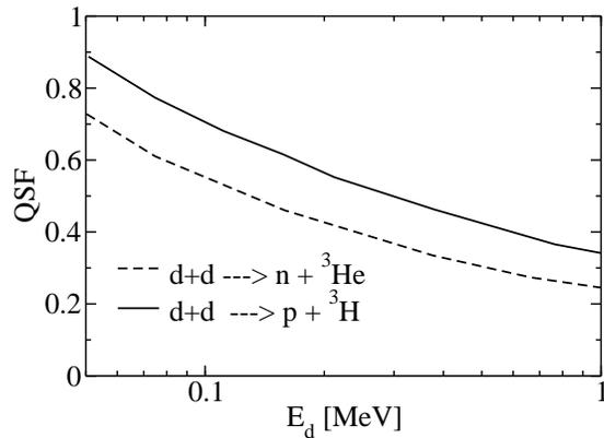
Figure 11: The quintet suppression factor (QSF) for  $d+d \rightarrow p+^3\text{H}$  and  $d+d \rightarrow n+^3\text{He}$  reactions as function of the deuteron energy in the laboratory system from an AGS calculation with the INOY04 potential [245].
