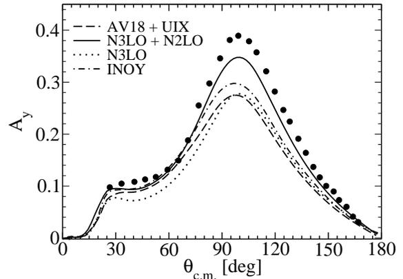
Figure 12:  $A_y$  of  $\bar{p}$ - $^3\text{He}$  scattering at  $E_p=4$  MeV calculated with various interactions. HH results [250]: AV18+UIX (dashed), I-N3LO+N2LO (solid); AGS results [243]: I-N3LO (dotted) and INOY (dash-dotted). Experimental data from Ref. [251].
