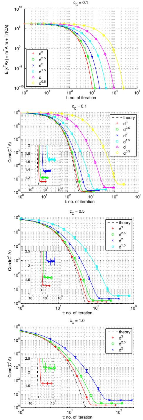
**Figure 1: Averages and standard deviations of the condition numbers  $\text{Cond}(C^t A)$  for  $c_C = 0.1, 0.5$ , and  $1.0$  and the expected objective function values for  $c_C = 0.1$ . Theoretical curves (26) of the condition number are also illustrated with dashed lines. All the lines are cut after first reach of the expected objective value to  $10^{-10}$ . Some results are omitted, for example  $n = d$  for  $c_C = 0.5$ , because numerically unstable computation occurs during search.**
