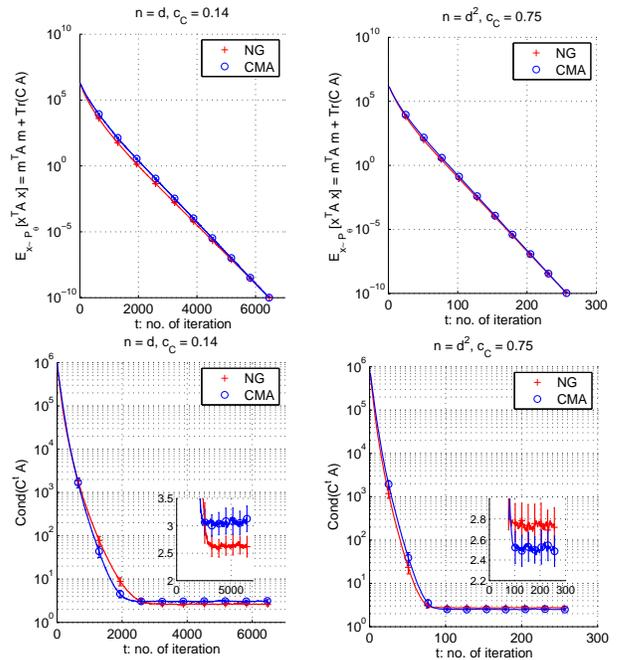
**Figure 3: Averages and standard deviations of the change of the condition numbers and the change of the expected objective function values for  $n = d$  and  $c_C = 0.14$  on the left, and for  $n = d^2$  and  $c_C = 0.75$  on the right. Other settings are the same as in Figure 1.**
