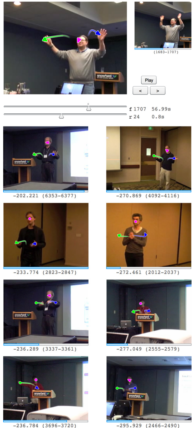
Figure 6. Gesture search by example. The user scrubbed through the top video until a suitable handwaving gesture was found then used this as the search input. The search returned the 8 closest matches.
