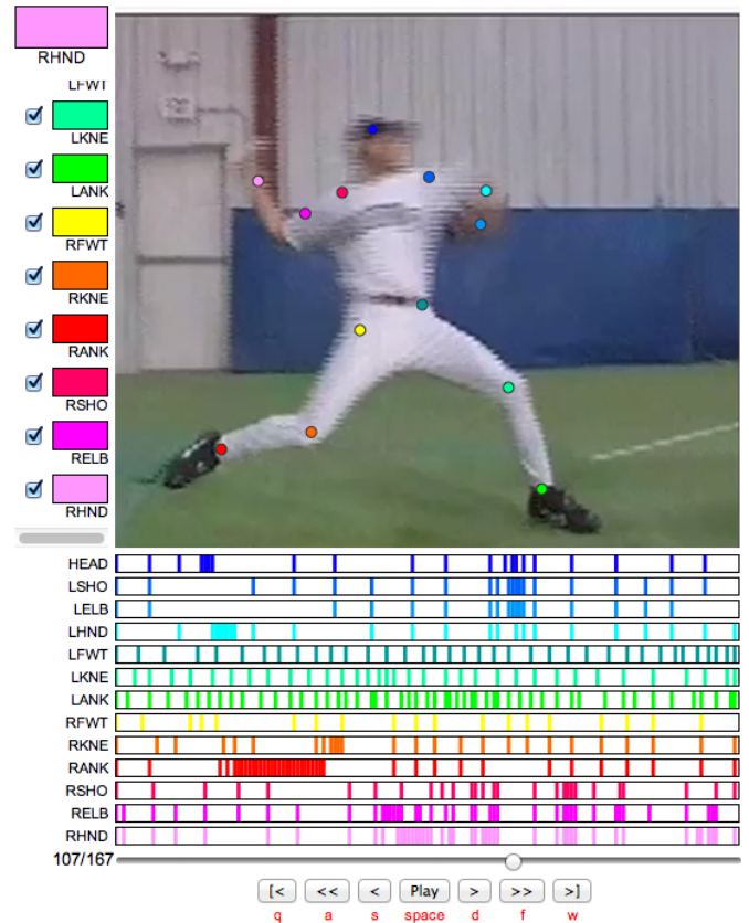
Figure 1. Our user interface for tracking, showing a completed 13-point baseball pitch annotation. Each marker and corresponding track is indicated with a different color. Tracks shows a line for every defined keyframe.
