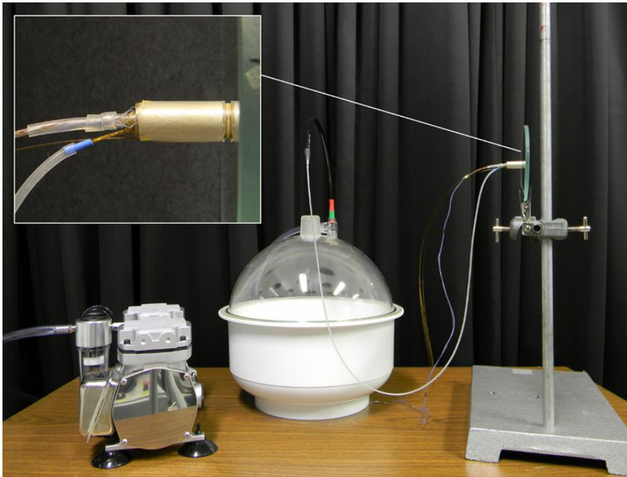
**Figure 5:** A demonstration of the new vacuum adhesion method, showing a single Starbug on a vertical glass surface
