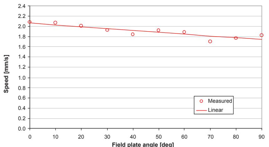
Figure 9: Plot of nominal Starbug speed vs. field plate angle for a ~0.5 m long fibre/wire bundle
