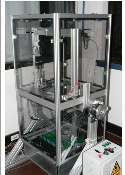
**Figure 6:** The Starbugs 'test rig' has control electronics and metrology for up to 20 Starbugs; in the centre of the enclosure is an interchangeable 400 mm diameter glass field plate
