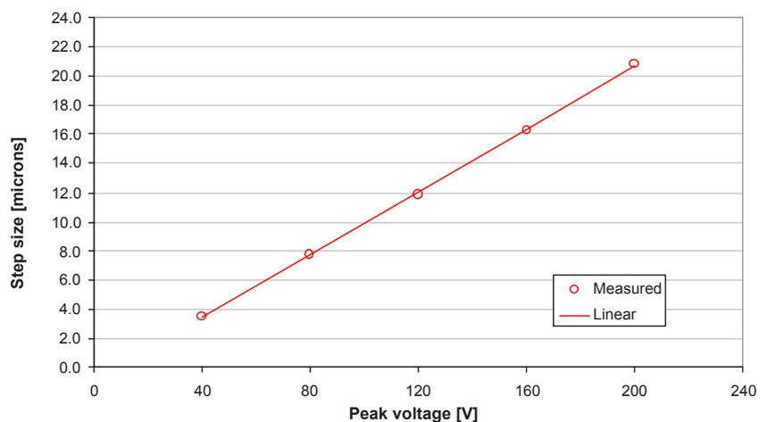
Figure 8: Plot of Starbug step size vs. waveform amplitude; results show an expected linear relationship
