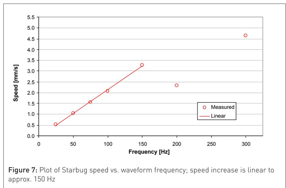
**Figure 7:** Plot of Starbug speed vs. waveform frequency; speed increase is linear to approx. 150 Hz
