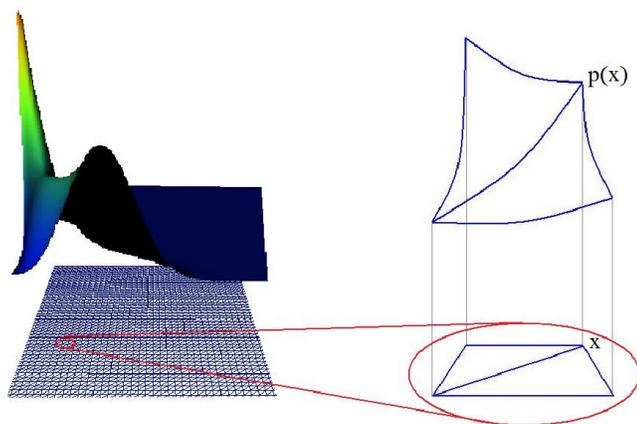
Figure 4.1: Finite elements construct a surface by combining simplices together. The quadratic elements used fit the function inbetween the mesh points with a quadratic formula.
