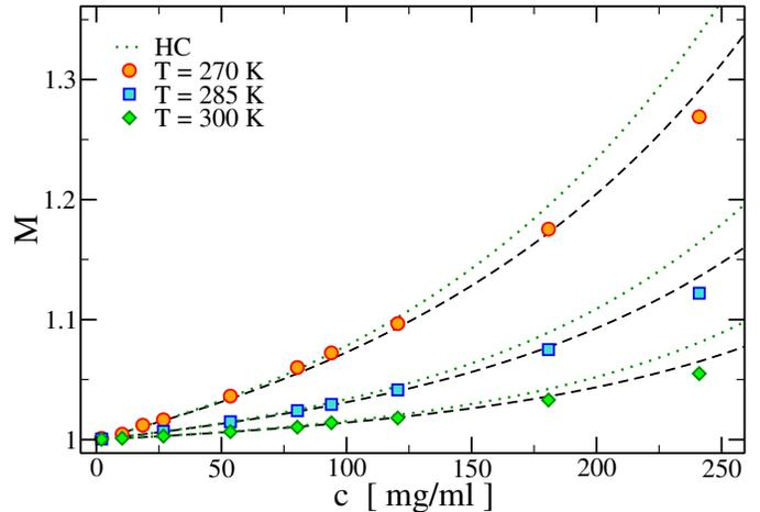
FIG. 5: Average chain length  $M$  in the isotropic phase at low concentration. Symbols are numerical results and dashed lines are theoretical predictions. Dotted lines are theoretical predictions using the excluded volume of HCs  $v_{excl}^{HC}$  (see Appendix B).
