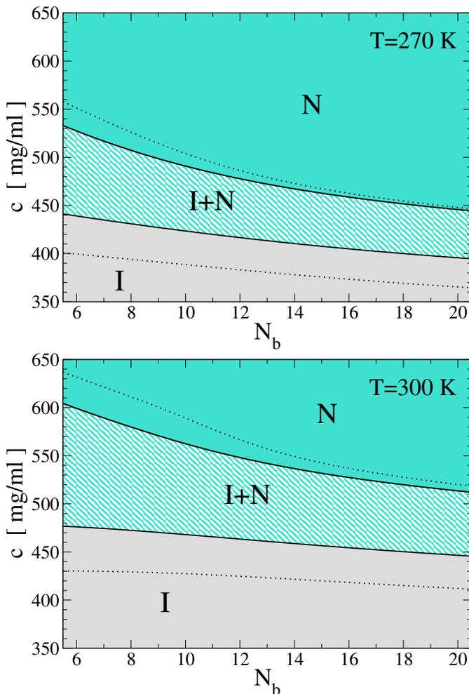
FIG. 6: I-N phase diagram in the  $c$  vs  $N_b$  plane for  $T = 270\text{ K}$  (top) and  $300\text{ K}$  (bottom). Dotted lines are theoretical phase boundaries calculated using the excluded volume of HCs  $v_{excl}^{HC}$  (see Appendix B).
