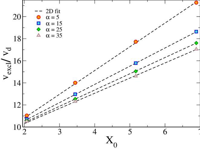
FIG. 10: Excluded volume as a function of aspect ratio  $X_0$  in the nematic phase together with analytic approximations for several  $\alpha$ . The dashed lines are obtained plotting the function reported in Eq. (9) and setting  $\eta_1 = 0.386419$ ,  $\eta_2 = 1.91328$  and  $\eta_3 = -0.836354$ .
