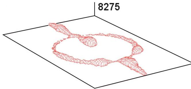
**Figure 10:** Fluid behavior on the larger junction pattern of Fig. 9 but with a *partially* wetting exterior ( $c_{\text{liquid,rock}} = 0.75$ );  $\theta_{\text{phil}} = 0^\circ$  and  $\theta_{\text{phob}} = 90^\circ$ . The other simulation parameters are the same as in Fig. 8. In this case droplets of liquid detach from the pattern and slide along the substrate.
