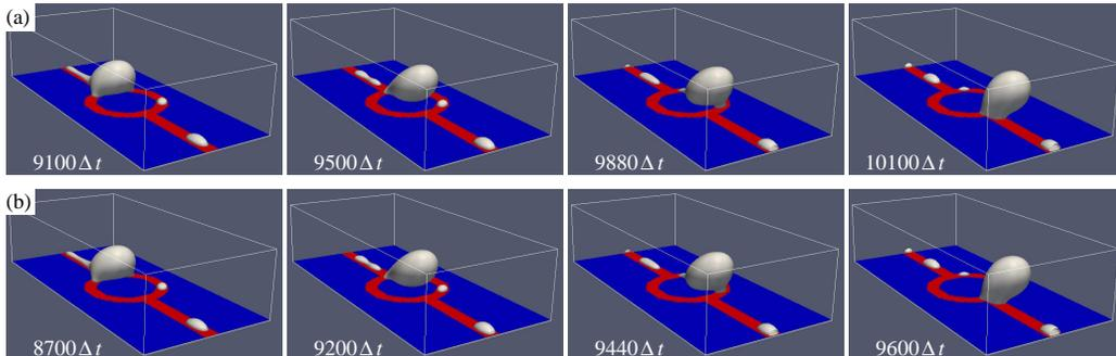
**Figure 5:** Simulation snapshots for  $\theta_{\text{phil}} \approx 80^\circ$ ,  $\theta_{\text{phob}} \approx 140^\circ$ , and  $v_{\text{shear}}/c_T = 0.17$  on a symmetric (a) and an asymmetric pattern (b). In the symmetric case the droplet is driven off the pattern, whereas in the asymmetric case it is still guided by the wider rear branch of the pattern.
