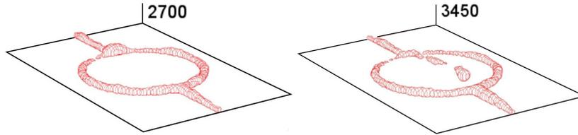
**Figure 9:** Behavior of a symmetrical junction pattern with twice the dimensions of Fig. 8. The other simulation parameters are the same as in Fig. 8;  $\theta_{\text{phil}} = 0^\circ$  and  $\theta_{\text{phob}} = 180^\circ$ . Liquid accumulates at the upstream node until its volume is too large to be held on the pattern by surface tension forces and a drop detaches and flies off.
