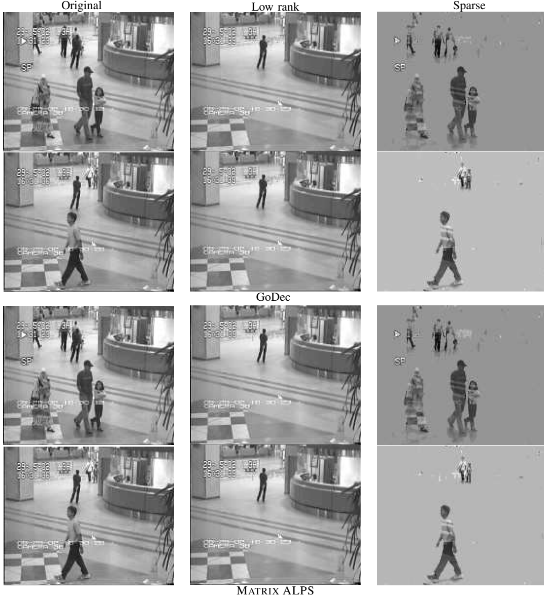
Fig. 2. Background subtraction in video sequence. Median execution times over 10 Monte-Carlo iterations. GoDec: 34.8 sec—MATRIX ALPS: 15.8 sec.
