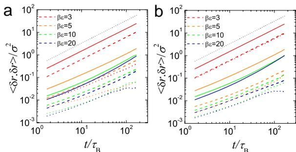
FIG. 7: **The effect of a quench times on the dynamics.** (a) Polydisperse system (b) monodisperse system. Mean squared displacement for quench depth and quench times. Solid lines - instantaneous quench, dotted lines, moderate ( $671\tau_B$ ) quench time, dashed lines, long ( $1.01 \times 10^4\tau_B$ ) quench time.
