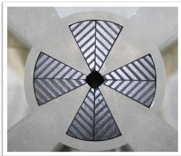
Figure 9: Detail of the magnet central part, the four poles in permendur and the PM blocks are clearly visible.
