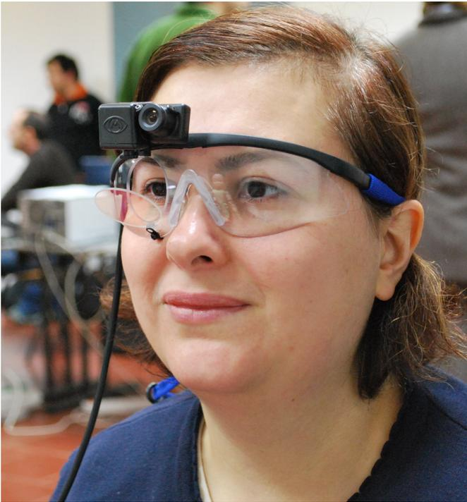
Fig. 2. The human interaction partner’s visual attention toward the robot is measured using a gaze tracking system.
