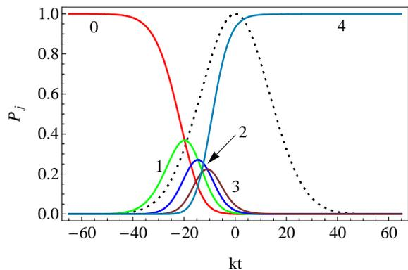
FIG. 2: (Color online) Dynamics of the photon number (indicated on the curves) distribution of the generated light. The atom is initially prepared in the state  $m_F = -2$ . The Gaussian pulse shape (26) is shown by a dotted line.
