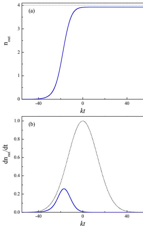
FIG. 3: (Color online) (a) Total number of output photons generated on the cycling  $5S_{1/2}(F=2) \rightarrow 5P_{3/2}(F'=3)$  transition of  $^{87}\text{Rb}$  atom and (b) corresponding flux in the units of  $k$ . The Gaussian laser pulse  $f_1(t)$  is shown by dotted line. For the parameters, see the text.
