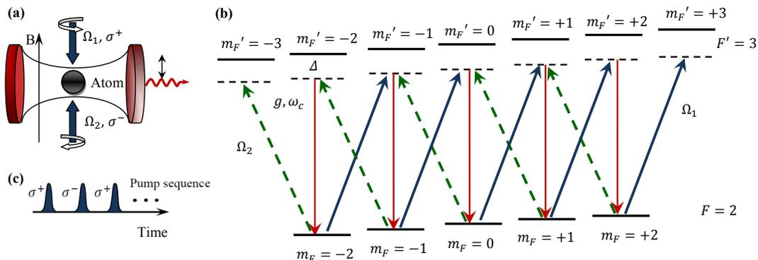
FIG. 1: (Color online) (a) Schematic setup. A single atom trapped in a high-Q cavity is driven by two laser pulses. (b)  $5S_{1/2}(F=2) \leftrightarrow 5P_{3/2}(F'=3)$  transition level structure of  $^{87}\text{Rb}$  in an external magnetic field.  $\Omega_1(\Omega_2)$  laser is shown by thick blue solid (green dashed) lines and the red thin solid lines show the cavity-mode coupling. (c) Sequence of laser pulses.
