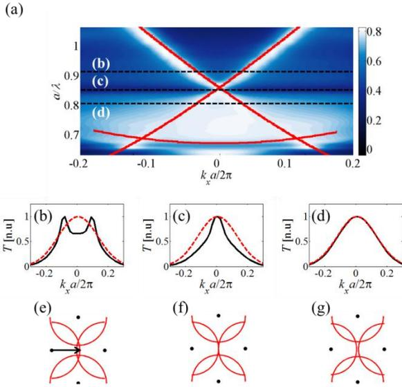
Fig. 5. (Color online) Normalized transmission functions of a rhombic GLMM along the  $\Gamma M$  direction. The solid red curves correspond to the crossing points of the nearest harmonics given by eq. 1, which intersect around the frequency 0.85. In figures (b), (c), (d) the far field distributions at D1 are plotted for frequencies below (0.82), close (0.85) and above (0.90) such point, as schematically represented in figures (e), (f) and (g).
