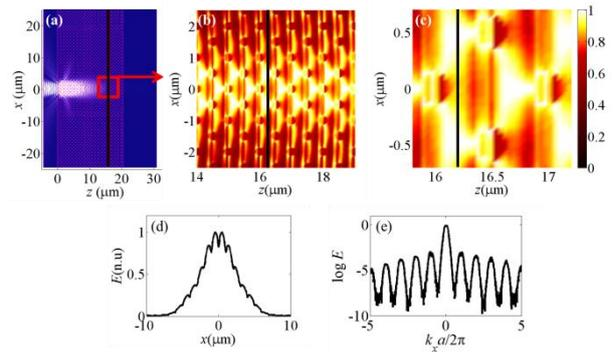
Fig. 2. (Color online) (a) Light beam propagation inside lossy GLMM with square lattice geometry, calculated by FDTD. The magnified view of the electric field shows the modulation of the propagated beam in the structure (b), and the shape of the Bloch mode (c). Vertical line D1 in figure (a) represents a plane at a distance  $z \sim 2 L_R$  used to reconstruct the angular transmission function. (d) Spatial distribution along the line D1 and (e) its Fourier transform.
