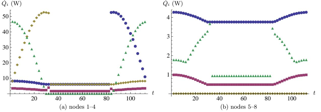
FIG. 4: Variation of the external heat input with time  $t$  (in minutes) along the orbit. For both plots, the node numbers are denoted by shape, in the order: dots (1,5), squares (2,6), diamonds (3,7), and triangles (4,8).
