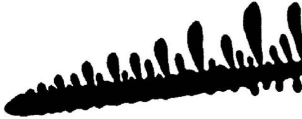
FIG. 4. Example of the crystal contour detection and the image binarization for the structure shown in Fig. 2 (160 sec).
