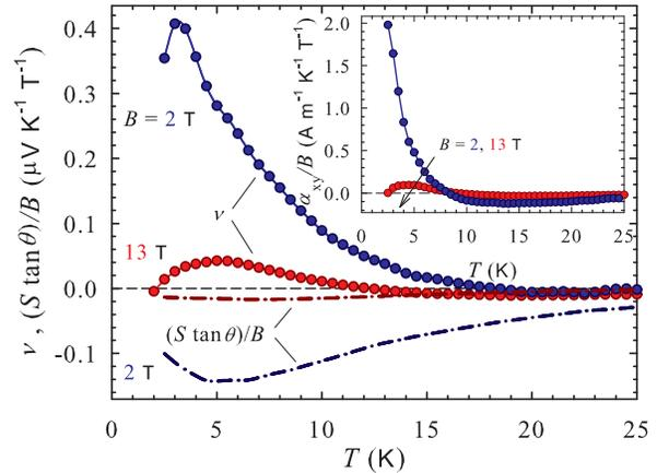
FIG. 2: (Color online) Temperature dependences of the Nernst coefficient (points) and  $(S \tan \theta) / B$  term (dash-dotted lines) in  $\text{Ce}_2\text{PdIn}_8$  measured at  $B = 2$ , and 13 T. Inset shows off-diagonal element of the Peltier tensor for the same magnetic fields and temperature range.
