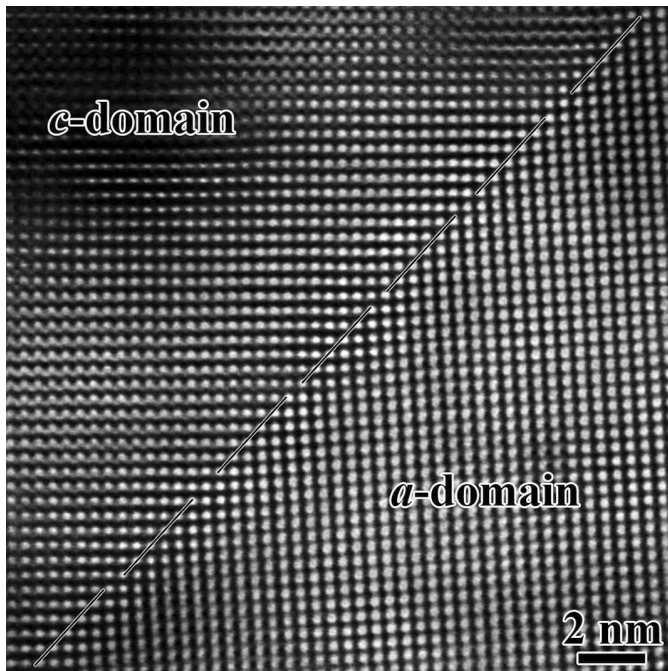
FIG. 2: A high-resolution TEM image of a PbTiO 3 thick film taken with an electron incident parallel to the [100] of PbTiO 3 . The 90° domain boundary is shown by the chain line.
