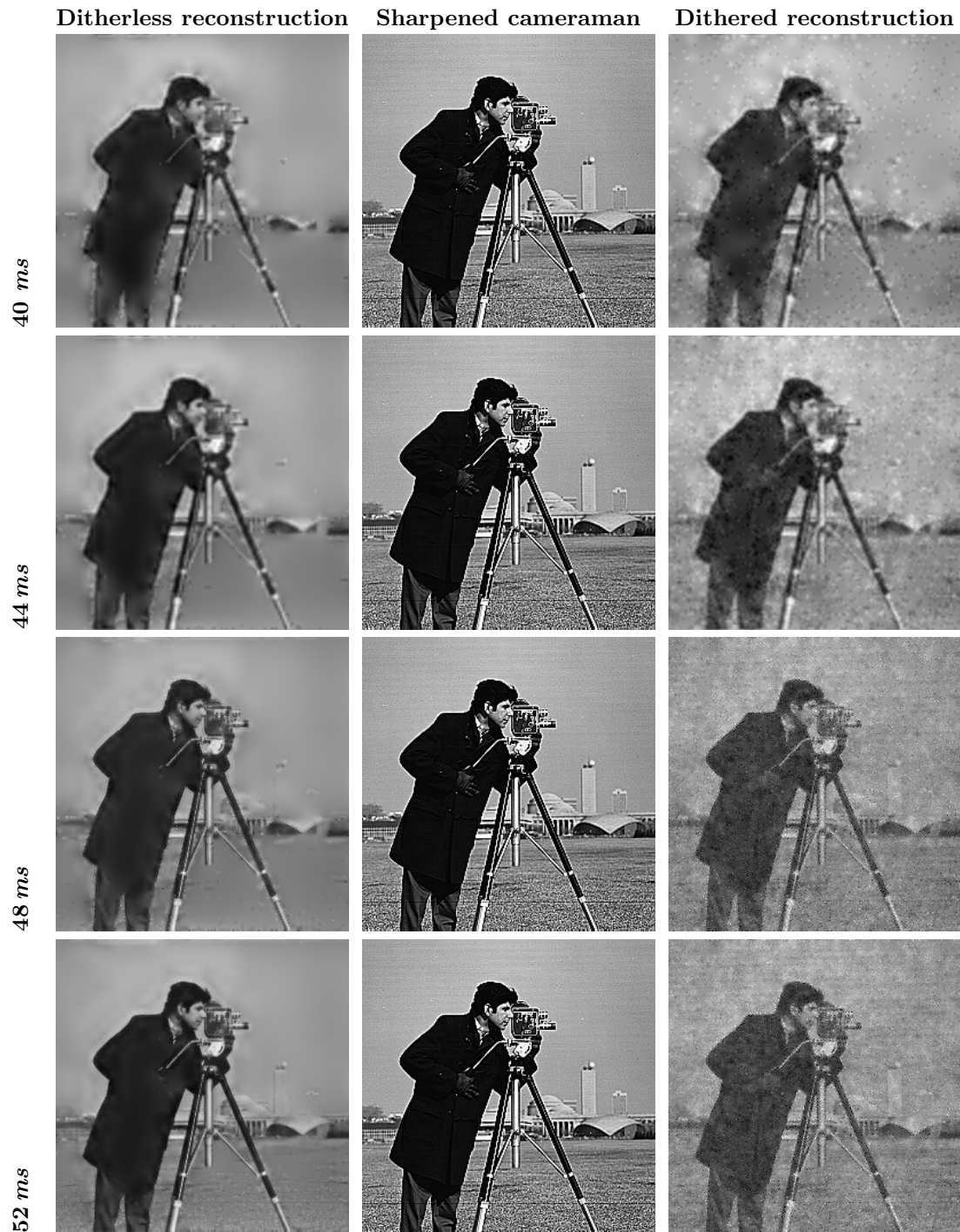
Figure 10: Perceptual impact of the multiscale dithering on the reconstruction of cameraman. The observation times t_{obs} are shown on the left. From top to bottom, t_{obs} take successively the values of: 40 ms, 44 ms, 48 ms, and 52 ms. The observation time shown in this figure is also the optimal observation t_{obs} = t_{obs}^* = 44 ms.
