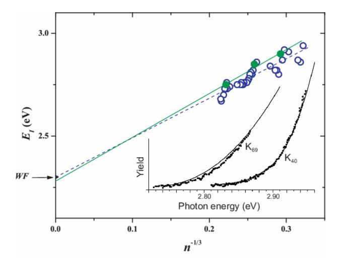
**Fig. 1.** Appearance energies of  $K_{30 \le n \le 101}$  clusters determined by a Fowler fit [11] to photoionization profiles [12]. With  $R=r_sn^{1/3}$  ( $r_s=4.86a_0$ ), linear regression gives  $E_I=2.30$  eV  $+0.34e^2/R$  for all points, or 2.29 eV+ $0.38e^2/R$  for the spherical closed-shell clusters. The potassium metal work function is 2.3 eV. Insert: examples of threshold data [12] and finite-temperature Fowler functions (solid lines) [11].
