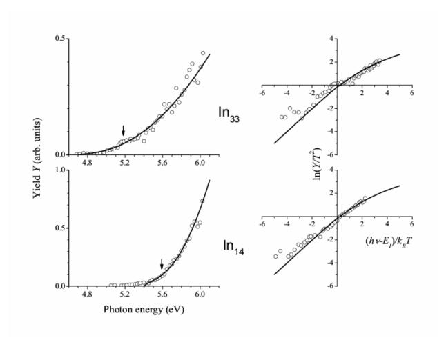
**Fig. 2.** Examples of Fowler fits for indium clusters (top:  $In_{33}$ , bottom:  $In_{14}$ ). On the right are Fowler plots following Eq. (1) (lines: finite-temperature Fowler functions, dots: experimental data [18]). On the left are the corresponding ionization threshold profiles (line: Fowler functions, dots: experimental data, arrows: deduced appearance energies  $E_I$ ).
