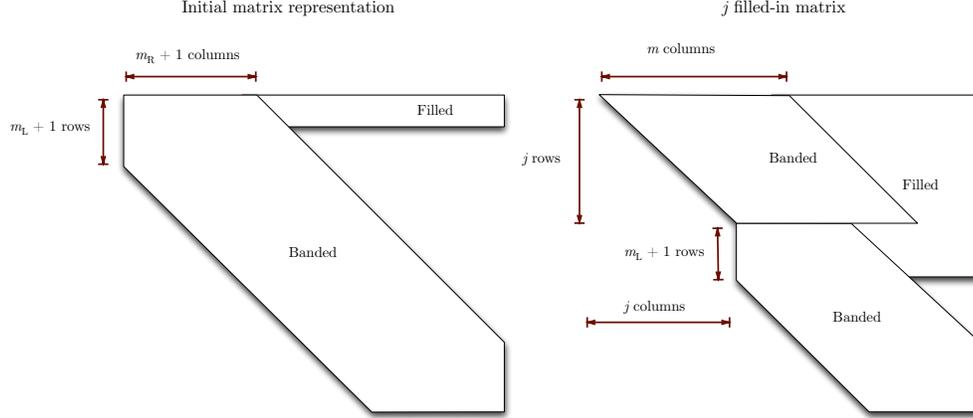
Fig. 5.1: Structure of operators during QR factorization. Left: Depicts the structure of the original differential operator. Right: Depicts a  $j$  filled-in matrix obtained after upper triangularizing the first  $j$  columns.
