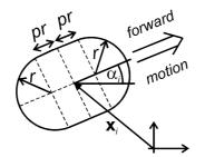
**Figure 13.** Rigid body model of an individual boat. The outline is composed of two semi-circles and two line segments
