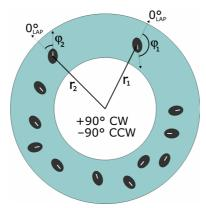
**Figure 3.** Schematic view of the pool with the boats. The local-angle polar (LAP) coordinate system defines the representation of the positions and orientations of the particles: r is defined as the distance from the center of the pool,  $\varphi$  is the angle between the local radial direction and the orientation of the boat.
