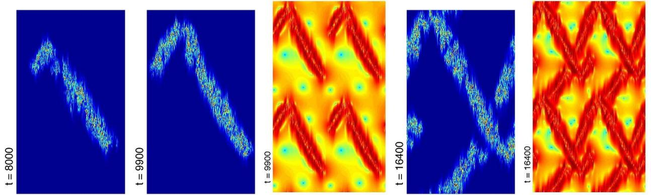
Figure 6: Formation of the chevron pattern and next the diamond. The central and right-most images display  $2 \times 2$  tilings of the local intensity of the mean in-plane flow corresponding to the images to their immediate left (decimal logarithms, color scale from blue ( $-10$ ) to yellow ( $-5$ ) to red ( $-1.7 = \log_{10} 0.02$ )).  $Re = 285$ . The streamwise direction is vertical.
