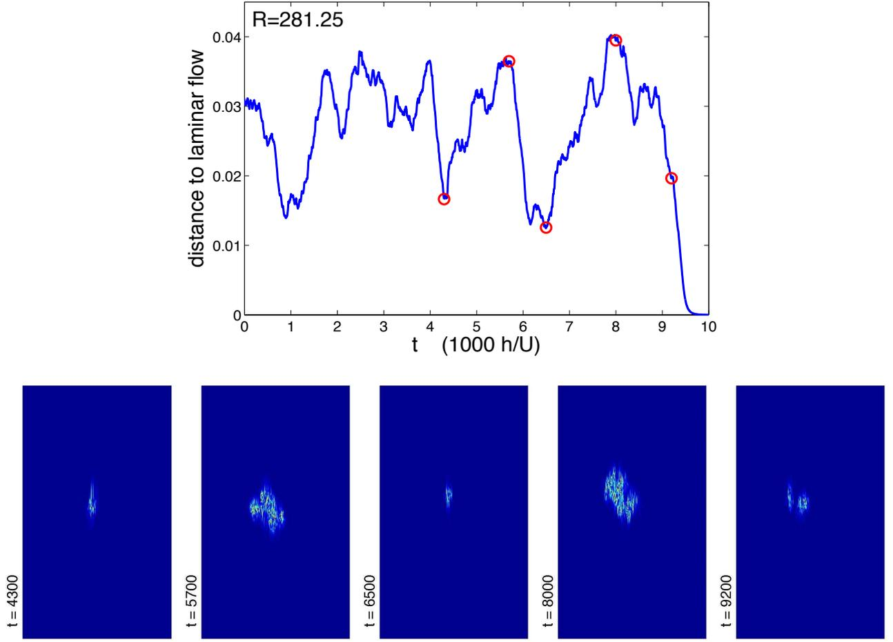
Figure 10: Decay of the germ for  $Re = 281.25$ . Top: Time series of the distance  $\Delta$  to laminar flow. Bottom: Snapshots of the solution at the instants identified by open circles ( $\circ$ ) in the graph. The streamwise direction is vertical.
