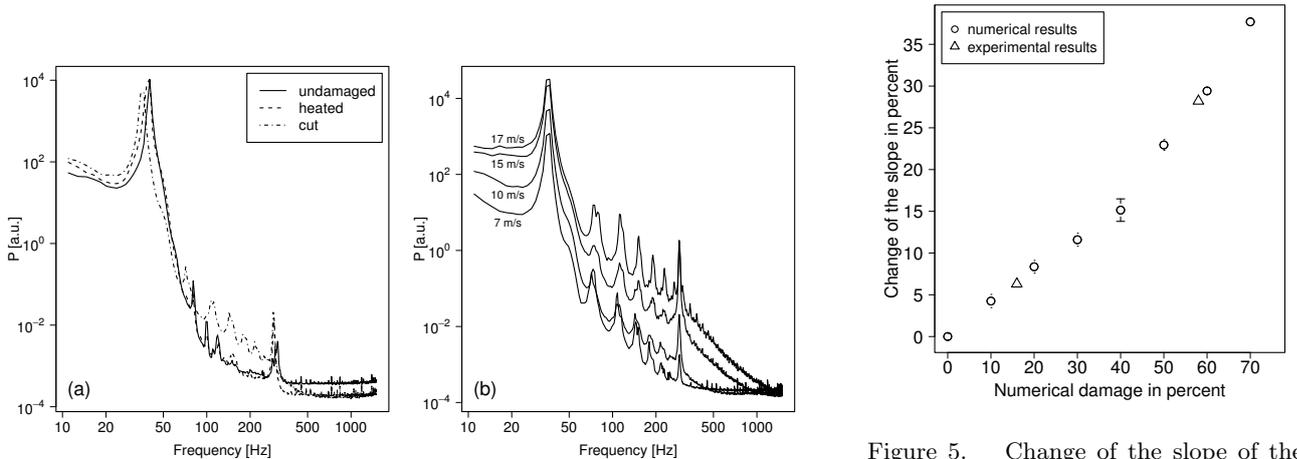
Figure 4. Power density spectra for the deflection signals in  $y$ -direction (a) at  $\bar{u} = 10$  m/s for different damages and (b) of the cut beam for different wind speeds.
