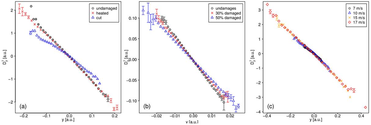
Figure 3. (Color online) Drift function in  $y$ -direction conditioned on  $x = 0$  (a) for three damages at  $\bar{u} = 10$  m/s (measurement), (b) for three damages (simulation) and (c) of the cut beam for different wind speeds.
