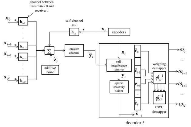
Figure 4. CCSM decoder for an  $i$ -th user.
