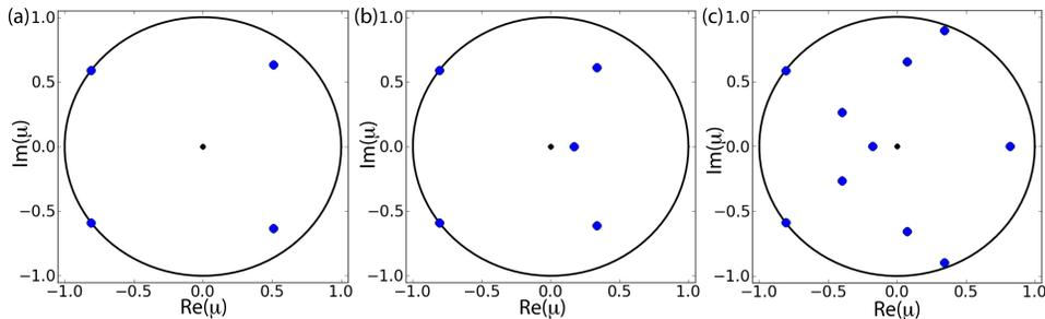
FIG. 4.2. Floquet multipliers  $\{\mu_i\}$  for overlapping pulses, i.e.  $M > 0$ : (a)  $J = 15$ ,  $M = 0$ , 2 neutrally stable eigenvalues; (b)  $J = 25$ ,  $M = 1$ , 2 neutrally stable eigenvalues; (c)  $J = 100$ ,  $M = 6$ , 2 neutrally stable eigenvalues. We have considered  $N = 5$  and  $T_s = 3.2$  ms.
