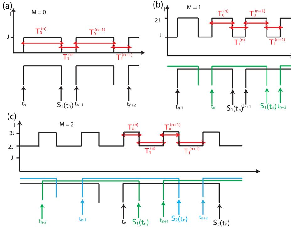
FIG. 3.1. PSPs in a splay state can overlap  $M$  times. (a) PSPs overlapping  $M = 0$  times (no overlaps); (b) PSPs overlapping  $M = 1$  times; (c) PSPs overlapping  $M = 2$  times. Independently of the value of  $M$  the synaptic current can take only two values in the time interval between two spikes: namely, during  $I(t_n < t < t_n + T_0^{(n)}) = (M+1)J$  and  $I(t_n + T_0^{(n)} < t < t_{n+1}) = MJ$ .
