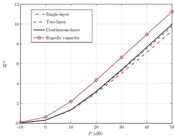
Fig. 2. The maximum throughput, the maximum two-layer expected-rate, the maximum continuous-layer expected-rate, and the ergodic capacity (all in *nats*) in the two-transmitter distributed antenna system.
