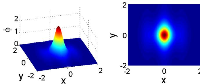
FIG. 4: (Color online) The same as in Fig. 3, but in the case of the Q1D linear potential (while the nonlinear potential remains two-dimensional), for  $g = +1$ ,  $q = 1$ , and  $\mu = -2.91$ ,  $N = 1.68$ . The shape of the solitons in the version of the model where the nonlinear potential is also made quasi-one-dimensional is quite similar to the present one.
