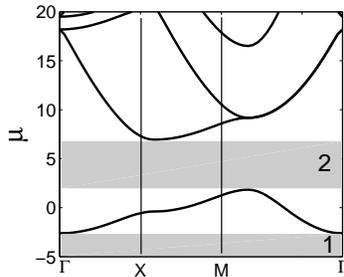
FIG. 1: The band structure of the linearized equation (1) in the first Brillouin zone, for depth  $\varepsilon = 7.4$  of the linear lattice;  $\mu$  is the chemical potential of the Bloch waves.
