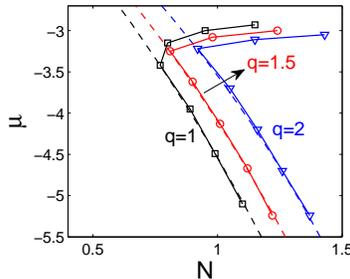
FIG. 2: (Color online) The chemical potential vs. the norm for soliton families in the semi-infinite gap of the model with the full 2D linear and nonlinear potentials, as produced by the VA (dashed curves), and as found from numerical solutions of Eq. (2) (chains of symbols).
