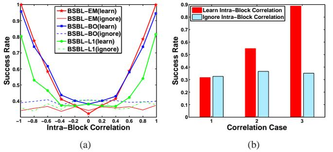
Fig. 2. (a) shows the benefit of exploiting the intra-block correlation. (b) shows the performance of BSBL-EM for three correlation conditions.
