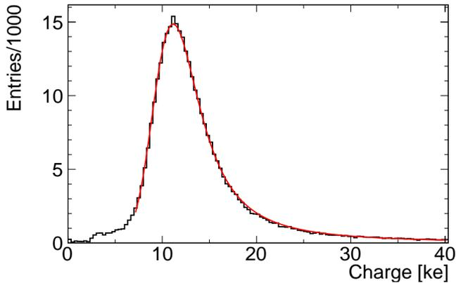
Figure 10: Charge collection distribution obtained from a  $^{90}\text{Sr}$  source measurement on sample E, irradiated up to  $5 \times 10^{15} \text{ n}_{\text{eq}}/\text{cm}^2$ , biased at 1000 V, and kept at an environment temperature of  $-60^\circ\text{C}$ . The distribution refers to all cluster sizes, and the measured MPV is  $(11 \pm 1)$  ke.
