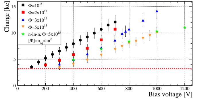
Figure 11: Charge collected by neutron irradiated modules, obtained from  $^{90}\text{Sr}$  measurements, as a function of the bias voltage. The modules were tuned to a front-end threshold of 3200 e. The uncertainties shown are due to the spread of the internal calibration capacitors. The results from the n-in-n modules are from [16].
