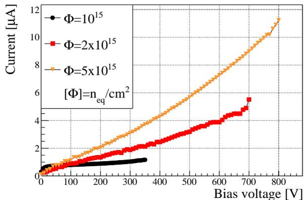
Figure 5: IV characteristics of the selected modules: B, C and E, irradiated up to 1, 2 and  $5 \times 10^{15} n_{\text{eq}}\text{cm}^{-2}$  respectively. The measurements have been scaled to a temperature of  $-20^\circ\text{C}$  [13].
