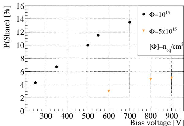
Figure 13: Dependence of charge sharing probability as function of the bias voltage for module B, irradiated up to  $1 \times 10^{15} \text{ n}_{\text{eq}}\text{cm}^{-2}$ , and E, irradiated up to  $5 \times 10^{15} \text{ n}_{\text{eq}}\text{cm}^{-2}$ , within the testbeam.
