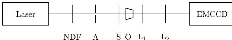
Figure 1. Schematic diagram for the experimental setup. NDF represents a neutral density filter, A is an aperture, S is the sample, O is a 20X objective,  $L_1$  and  $L_2$  are two collimating lenses. EMCCD is an Electron-Multiplying Charge Coupled Device for collecting the images.
