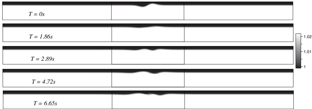
Figure 3: Density field from the numerical simulation of the evolution from the initial data in the 1232 cm long tank with the center 308 cm test section marked by the vertical lines.
