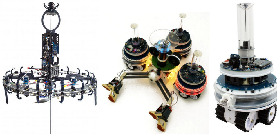
Figure 7 Photos of swarmanoid eye-bot (left), hand-bot being carried by three foot-bots (center) and foot-bot (right).
