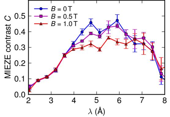
Figure 6: Contrast of the MIEZE signal in the direct beam for various magnetic fields at the sample position. The small loss of  $C$  with increasing field is due to the missing coupling coils and the insufficient  $\mu$ -metal shielding.
