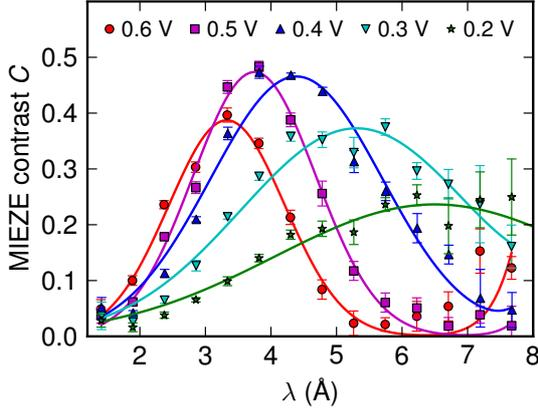
Figure 3: Contrast as a function of wavelength in the direct beam for various output voltages applied at the RF generator. The solid lines are guides to the eye. The MIEZE frequency was  $\Delta f = 25$  kHz. Note that with eq. (2) half the RF field should flip twice the wavelength; this does not hold for the output voltage due to nonlinearities in the RF amplifier and circuit.
