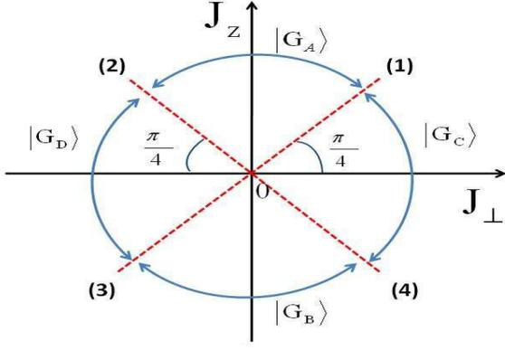
FIG. 8: (Color online) The quantum ground states in all the parameter regimes.  $|G_i\rangle$  ( $i = A, B, C, D$ ) represent the ground states in the four bulk regimes, and are given in Secs. VIIIA to VIIID. (1) to (4) represent the four boundaries, in which the ground states are described in Sec. VIIIE.
