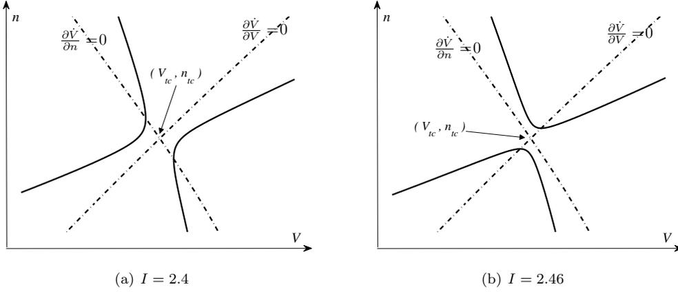
Figure S5: **Phase portrait of the model for different values of the input current in the presence of calcium channels.** The  $V$ -nullcline is drawn as a solid line. The dashed-lines depict the locus  $\frac{\partial f_V}{\partial V} = 0$  and  $\frac{\partial V}{\partial n} = 0$ , respectively.
