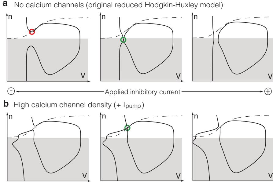
**Figure 3: Unfolding of the transcritical bifurcation in the global reduced Hodgkin-Huxley phase portrait.** (a and b) Phase portraits of the original reduced HH model without (a) and with a calcium current (b). A constant inhibitory current of increasing amplitude (from left to right) is applied to the model. The transcritical bifurcation is non physiological in the classical reduced HH model (a) but plays an important physiological role in the presence of calcium channels (b).
