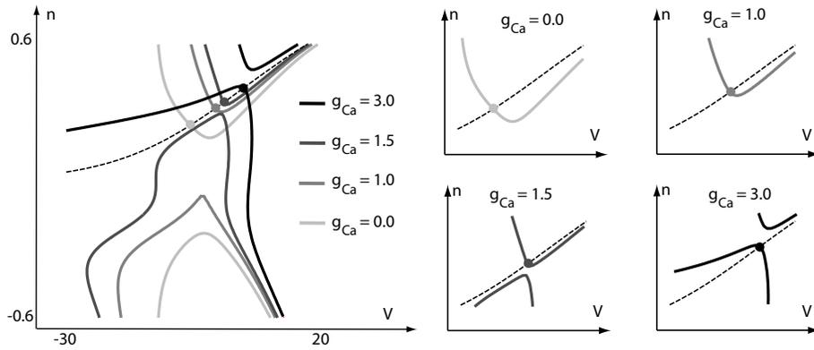
Figure S3: Nullcline intersections in the reduced model (5) with calcium current for different values of the calcium conductance. The  $n$ -nullcline is depicted as a dashed line, the  $V$ -nullcline as a solid line. The associated calcium conductance is expressed via a gray scale, as indicated in the figure legend. The calcium pump currents is given by  $I_{Ca,pump} = 0.0, -0.74, -2.78, -15.6$  for, respectively,  $g_{Ca} = 0.0, 1.0, 1.5, 3.0$ .
