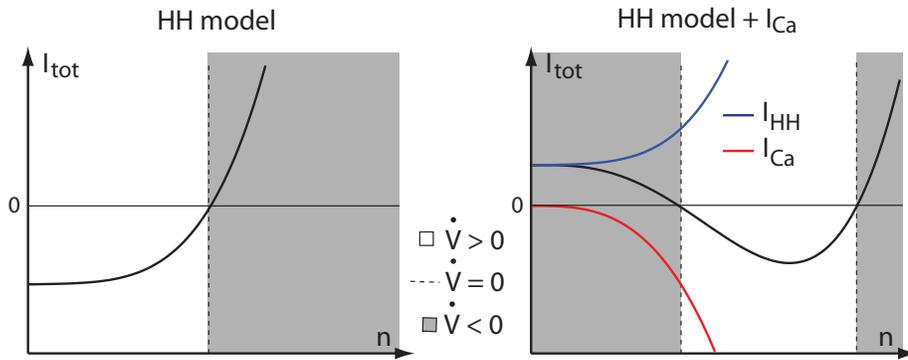
Figure S2: **Total ionic currents for  $V$  fixed as a function of  $n$  without (left) and with calcium channels (right).** Blank portions corresponds to the values of  $n$  where  $\dot{V} > 0$ , shaded portions corresponds to the values of  $n$  where  $\dot{V} < 0$ , and the dashed lines correspond to the values of  $n$  where  $\dot{V} = 0$ . Note that the total ionic currents monotonically increase only in the absence of calcium channels (left).
