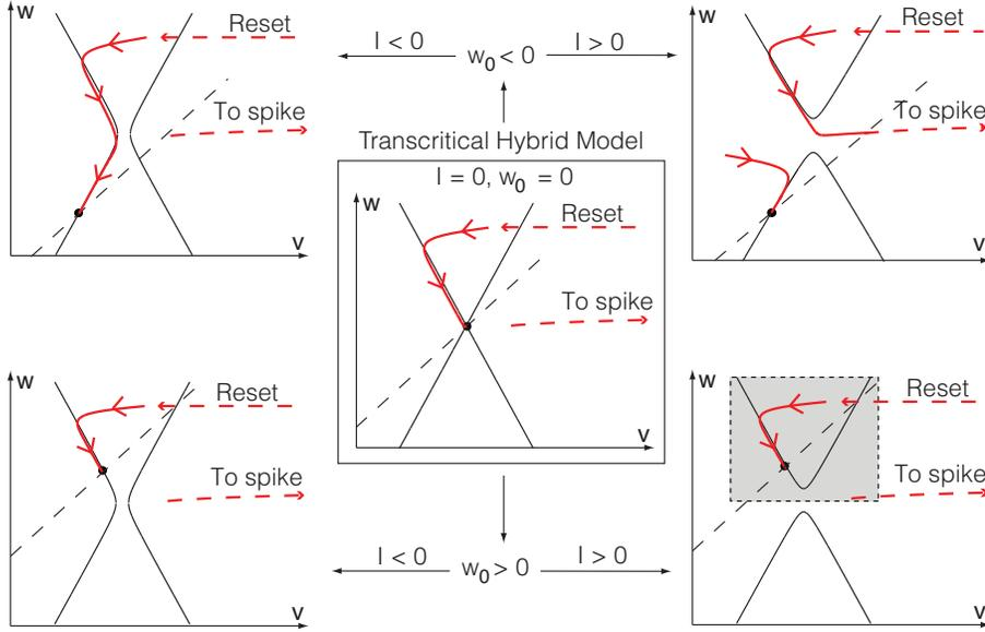
**Figure 4: Schematic phase-portraits of the transcritical hybrid model for different values of  $I$  and  $w_0$ .** The  $v$ - and  $w$ -nullclines are drawn as full and dashed lines, respectively. The trajectories are drawn as red oriented lines. Many different phase-portraits derive from the transcritical hybrid model, including the one of the fold hybrid model, which only captures the shaded area.
