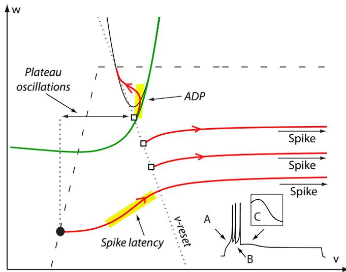
Figure S10: **Phase portrait and voltage time course (inset) of the Izhikevich model of TC neurons.** The trajectory is depicted as a solid oriented red line. The  $v$ -nullcline is depicted a solid line, the  $w$ -nullcline as a dashed line. The point line sketches the  $v$ -rest law. The stable manifold of the saddle point is depicted as a green line. Parameters as in [4, Sections 8.3.1].
