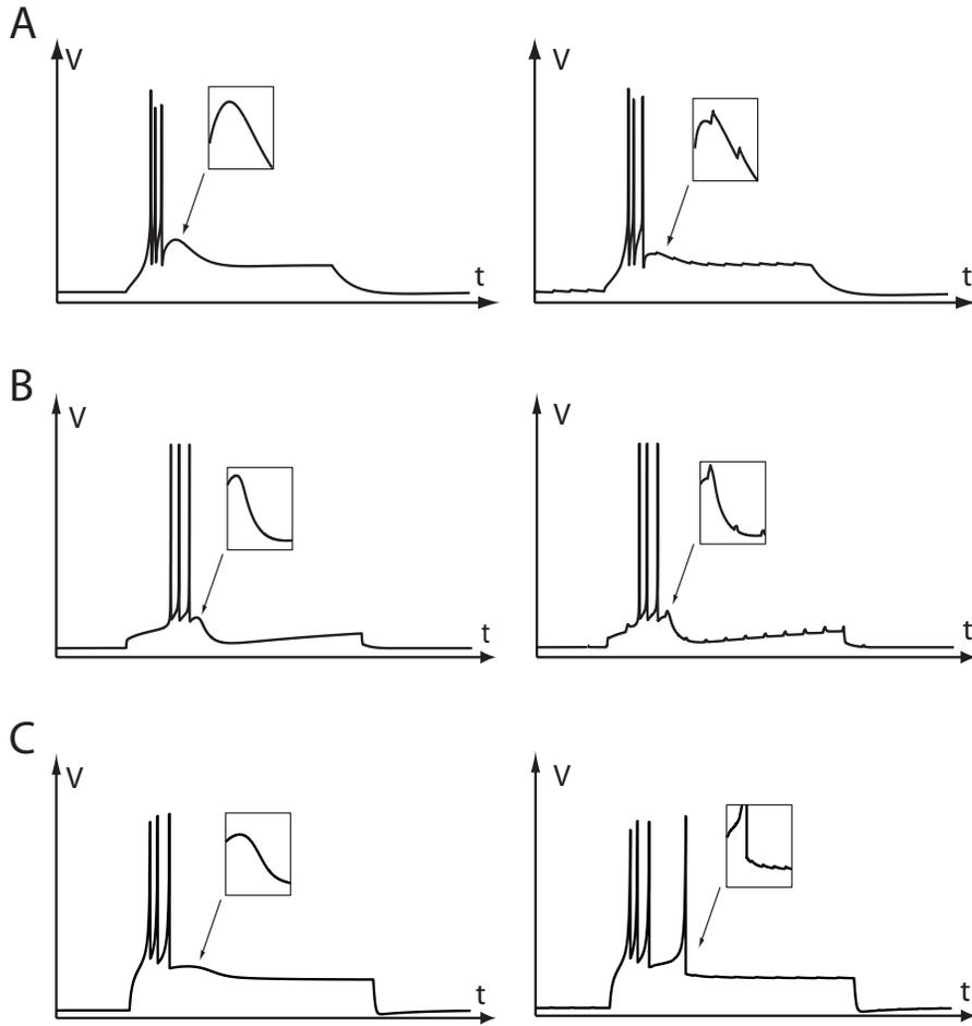
Figure S11: Nominal step response (left) and step response in the presence of small current pulses in the 200 compartments TC neuron model (a), the proposed hybrid model (b), and the Izhikevich model of TC neuron ([5, Section 8.3.1]) (c).
