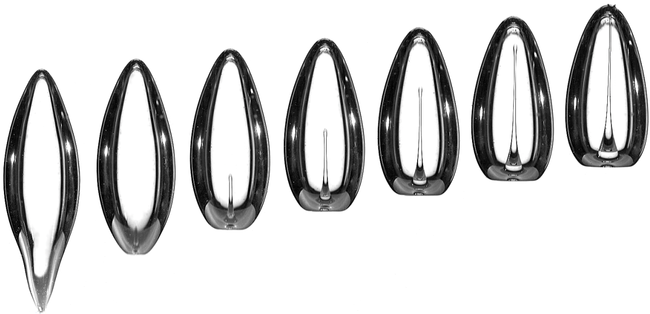
FIG. 1. Time sequence of the jet developing inside a large bubble just after its release from a submerged nozzle. The large bubble pinches off at the first image and the back-to-equilibrium dynamics exhibits an intense and concentrated jet. The time lapse between the snapshots is \Delta t = 3 ms. The bubble height, right after detachment, is H = 4.22 cm, the bubble front velocity is V_{\text{front}} = 0.67 m.s ^{-1} and the jet velocity is V_{\text{jet}} = 2.69 m.s ^{-1} . The liquid viscosity is \mu = 420 mPa.s. The gas is injected through an injector of diameter d = 1.8 mm at an airflow rate of Q = 4.4 \ell .min ^{-1} . The fluid height is h = 10 cm.
