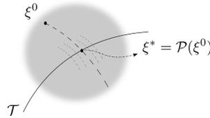
Fig. 5: Geometric representation of the trajectory manifold: every point of  $\mathcal{T}$  is a trajectory of the system. The projection of the curve  $\xi^0 = (\alpha(\cdot), \mu(\cdot))$  on  $\mathcal{T}$  through  $\mathcal{P}$  is the trajectory  $\xi^* = (\mathbf{x}(\cdot), \mathbf{u}(\cdot))$ .
