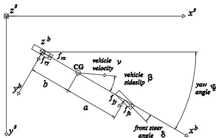
Fig. 1: LT-CAR model. The figure show the quantities used to describe the model.
