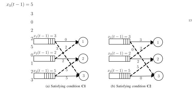
Fig. 5: Examples of balancing server reallocations (the weight  $c_{n,k}(t)x_n(t-1)$  of each edge (n,k) is also shown)
