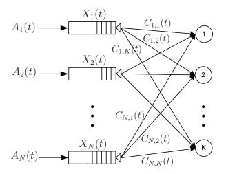
Fig. 2: Discrete-time MQMS-Type2 system with N parallel queues and K servers.
