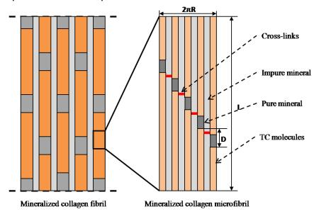
**Figure3**. Illustrated in plans of mineralized collagen fibril and unfolding in plane of repetitive portion of mineralized collagen microfibril structures. The model consists of three phases: (i) TC molecules, (ii) pure mineral: crystalline hydroxyapatite located within gaps created by the TC assembly; (iii) impure mineral: water, crystalline hydroxyapatite and porosity (light grey). Cross-links are connecting the TC molecules.
