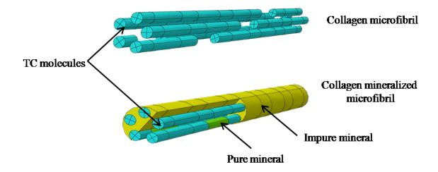
Figure 4. Proposed 3D FE model of mineralized collagen microfibrils
