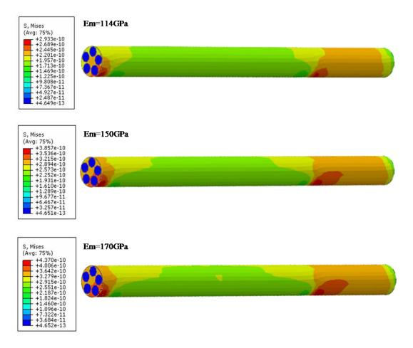
**Figure9.** FE Von Mises stress contours under varying mineral Young's modulus at Ec=2.7GPa and N=0.
