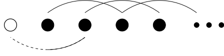
FIGURE 2. Visualisation of (5): the bond at the bottom of the graph is counted half in the Cauchy–Born model, even though it does not exist in the atomistic model, hence it gives a contribution -\frac{1}{2}\phi(2y'(0)) to the surface energy.
