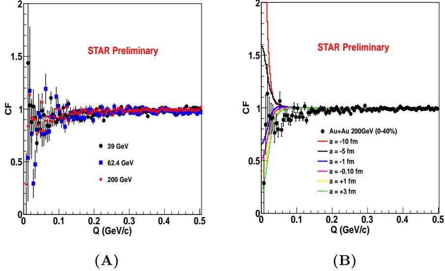
Fig. 2. (A) The purity corrected  $\Lambda\Lambda$  correlation function from 0-40% most central Au+Au collisions at  $\sqrt{s_{NN}} = 39$  (circle), 62.4 (square) and 200 (star) GeV. (B) The  $\Lambda\Lambda$  correlation function from 0-40% most central Au+Au collisions at  $\sqrt{s_{NN}} = 200$  GeV with theoretical correlation function for a Gaussian source of size  $R_x = R_y = R_z = 4$  fm for different scattering length (a).
