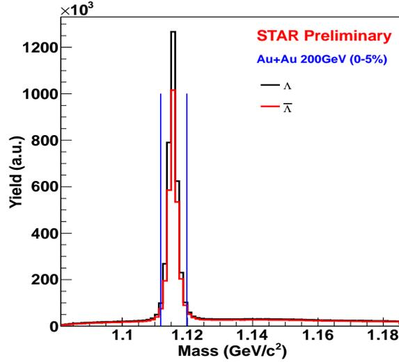
Fig. 1. The invariant mass distribution for  $\Lambda(\bar{\Lambda})$  from 0-5% most central Au+Au collisions at  $\sqrt{s_{NN}} = 200$  GeV. The  $\Lambda(\bar{\Lambda})$  candidates falling in the mass range 1.112 to 1.12  $\text{GeV}/c^2$ , shown by blue lines, were selected for the correlation measurement.
