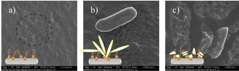
Fig. 3. SEM images illustrating each step of the experiment (a) step 1- phages are immobilized on the fiber core surface, (b) step 2 – capturing of *E.coli* bacteria by the phages, and lysis of the bacteria (c) step 3 - fiber is washed with PBS, bacteria chunks remain bound to the core surface.
