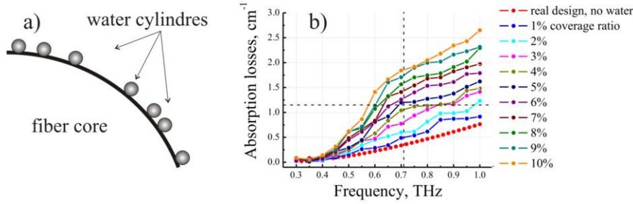
Fig. 90. (a) Randomly distributed 1  $\mu\text{m}$  water cylinders on the waveguide core's surface for a given value of surface coverage. (b) Absorption loss of the fundamental mode for the fiber with a bacteria layer as a function of the bacteria coverage ratio. The crossing of the dash lines in the figure corresponds to the experimentally measured value of the propagation losses minus the theoretically estimated coupling loss for the  $10^9$  cfu/ml concentration of bacteria.
