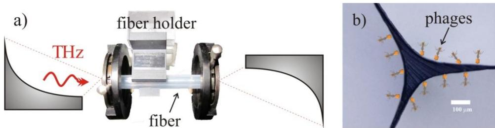
Fig. 2. (a) Schematic of the experimental setup: fiber is placed between the focal points of the two parabolic mirrors, (b) schematic presentation of phages adsorbed onto the fiber core. The capsid adsorbed onto the fiber, while the tail (which is specific to the bacteria) faces towards the cladding for bacteria capturing.
