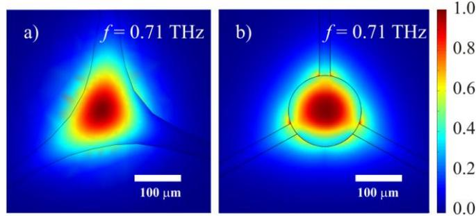
Fig. 9. Transverse distribution of power flow for the fundamental mode of (a) the real waveguide and of (b) the simplified design of the waveguide profile. The field is confined in the central solid core and is guided by total internal reflection.
