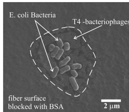
Fig. 5. Zoom-in of the waveguide core, dashed line marks the area covered with bacteriophages. Bacteria are clustered in the phage-covered surface with the rest of the surface blocked by BSA.
