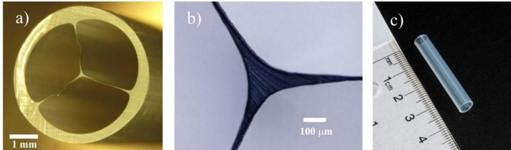
Fig. 1. (a, b) The THz fiber featuring a 150  $\mu\text{m}$  core suspended by three 20  $\mu\text{m}$ -thick bridges in the center of a 5.1 mm diameter tube, (c) 4 cm-long fiber piece used in the experiments.
