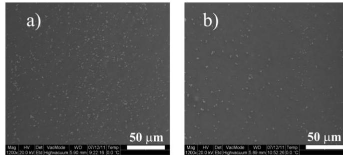
Fig. 8. SEM images of the fiber core with bacteria concentration of (a)  $10^9$  cfu/ml and 10 min interaction time (b) with a concentration of  $10^6$  cfu/ml, 10 min interaction time.
