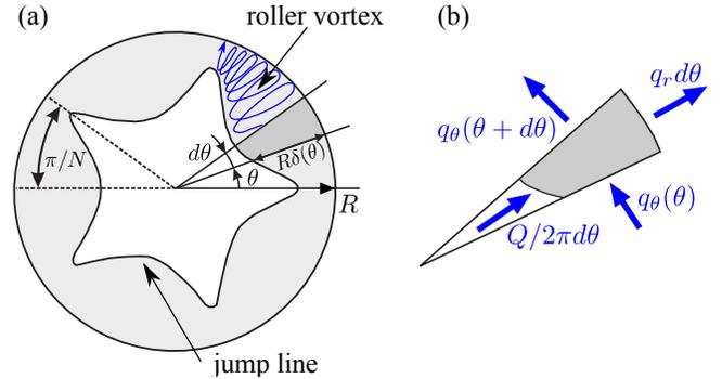
FIG. 7. (Color online) (a) Schematic top view of a pentagonal jump. The gray shaded wedge represents the control volume with infinitesimal angle  $d\theta$ , also seen in Fig. 6. (b) Enlargement of the wedge-shaped control volume. Arrows (blue) represent the radial and tangential mass flux  $q_r$  and  $q_\theta$ , i.e. the flux in and out of the control volume.
