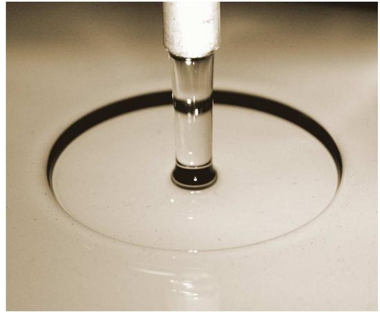
FIG. 1. Circular hydraulic jump. A cylindrical jet of fluid impinges vertically on a horizontal glass plate and forms a circular hydraulic jump. The fluid used here is ethylene glycol (about 10 times the viscosity of water).
