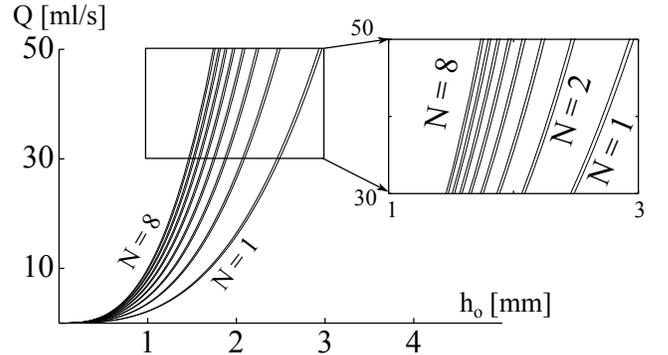
FIG. 12. Bifurcation diagram in physical parameters  $(h_o, Q)$ . The regions in which polygonal solutions with each  $N$  up to  $N = 8$  are shown. The  $h_o$ - $Q$  relationship for the border curves, especially in the enlarged inset, is qualitatively similar to the measured FIG. 5 despite quantitative disagreement. The bands are predicted to be thinner and do not overlap in the model, unless  $N \geq 22$ , unlike in experimental observations.
