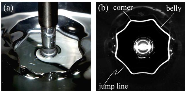
FIG. 2. Polygonal jump with eight corners. (a): Top view from an oblique angle. (b): View from below through a glass plate. The jump line becomes visible by diffracting light shone on the jump from above. The “belly” between two corners (or “necks”) is where the roller is thickest.
