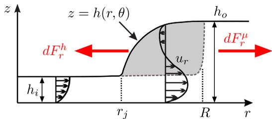
FIG. 8. (Color online) Side view of the wedge in Fig. 6. The height inside and outside of the jump are  $h_i$  and  $h_o$ , respectively. We treat the roller eddy (shaded region) as a separate body of fluid from the main stream, and assume the force balance of the hydrostatic force  $dF_r^h$  and the shear force  $dF_r^\mu$  in the radial direction (forces indicated by bold red arrows).
