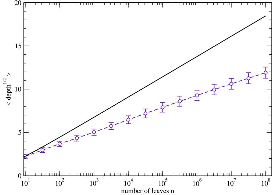
Figure 8: Depth as a function of tree size  $n$  for the innovation model ( $\circ$ ) and for the deterministic growth (solid curve) according to Equation (15). Note that square root of depth is plotted such that a straight line in the plot indicates a depth scaling  $d(n) \sim (\log n)^2$ . For each size  $n$ , the plotted point ( $\circ$ ) is the average over  $\sqrt{d(n)}$  for 100 independently generated trees. Error bars give the standard deviation.
