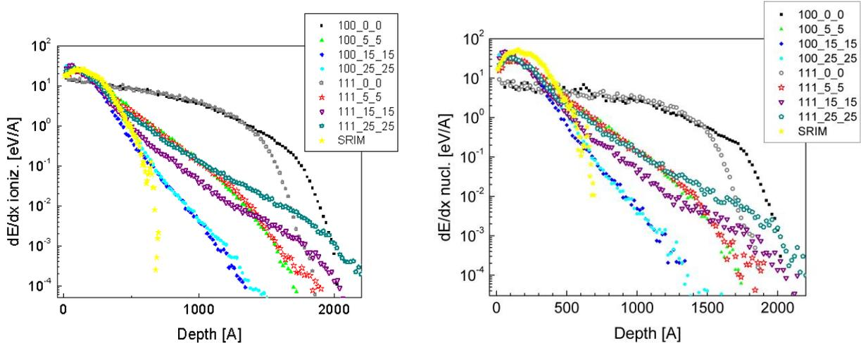
Figure 3: Depth dependence of the electronic (left) and nuclear (right) energy loss of a 15 keV selfrecoil in silicon, with the indication of the tilt and rotation angles of the direction of the particle for crystalline targets.
